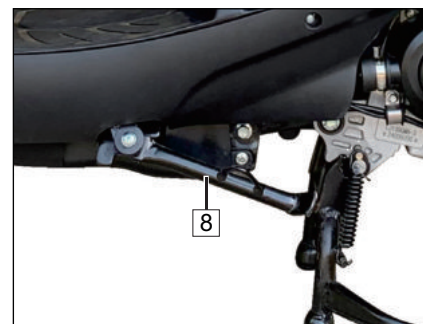
4. Fault diagnosis tester (6). 5. The ignition key(7) at "↻" position. 6. Side (8) switch at horizontal position.
