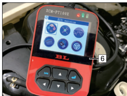
4. Fault diagnosis tester (6). 5. The ignition key(7) at "↻" position. 6. Side (8) switch at horizontal position.
